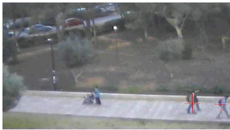
Figure 4: Imperfect pedestrian tracking example. The left pedestrian is detected together with the stroller and is discarded due to non-legitimate height-width ratio.
